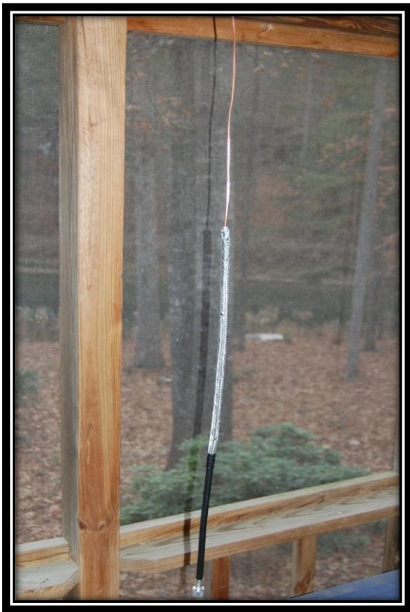
Figure 4. Example of VHF Coaxial Sleeve Antenna
